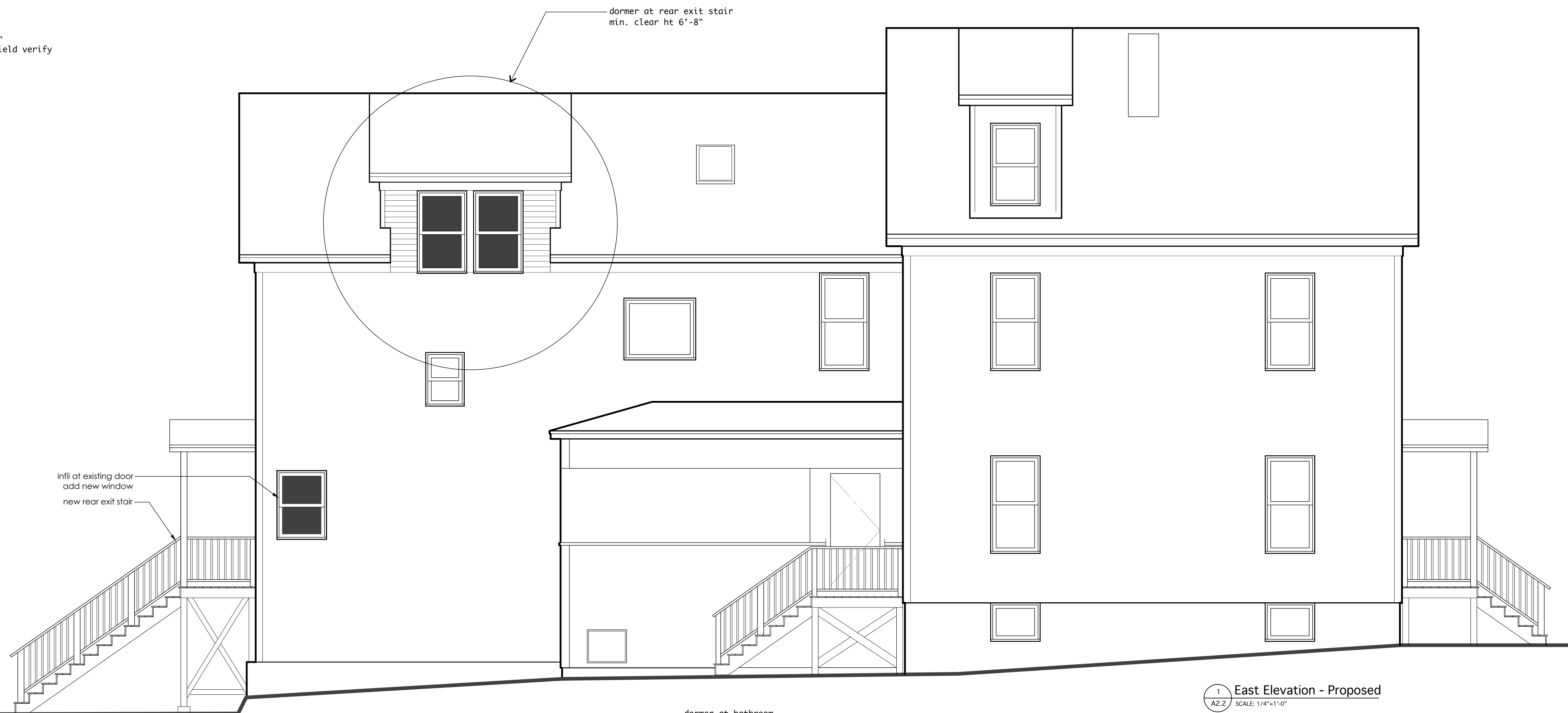
3 Proposed Rear Stair Dormer (Front similar) A2.0 SCALE: 1/4"=1'-0"
