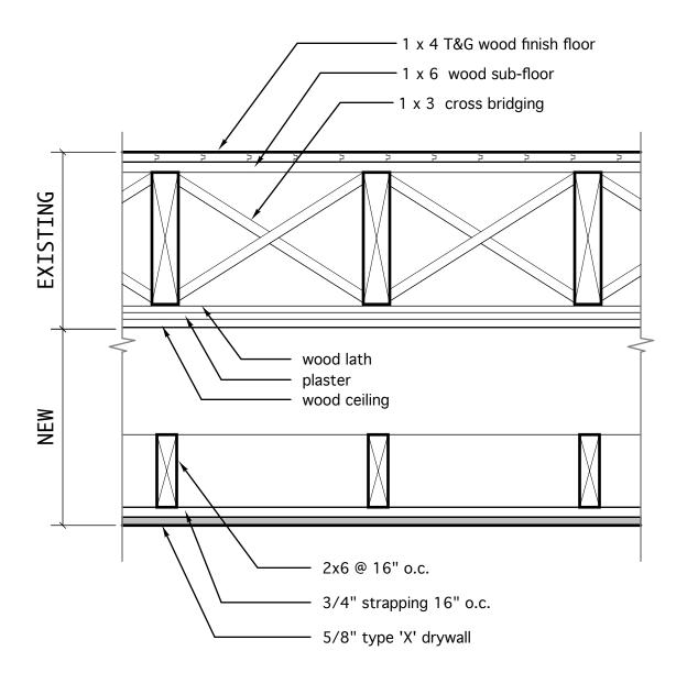
1 Hr. Fire Rated Detail for First floor Ceiling based on UL Design No. L522
