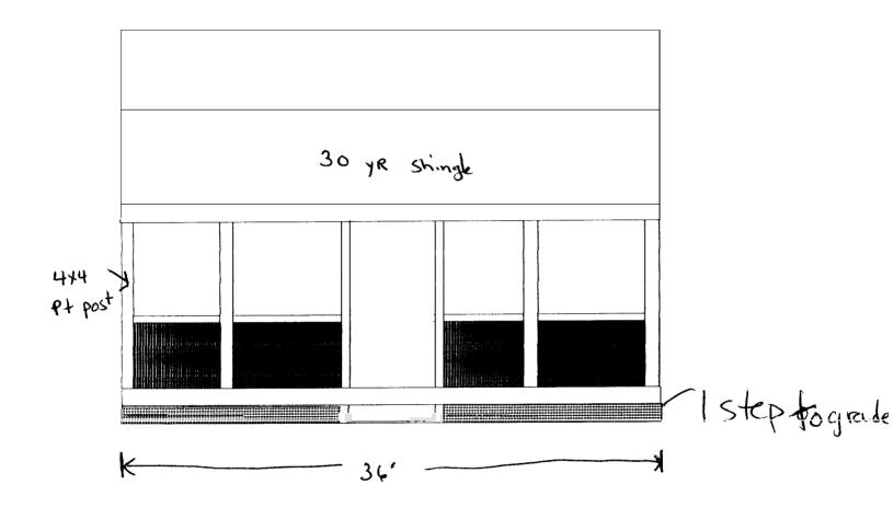
Porch Rafters: 2x8x14 16" oc Roof: 5/8 05B 4x8 Header: 3-2x6x12 Laminated Together Railing: Vinyl
