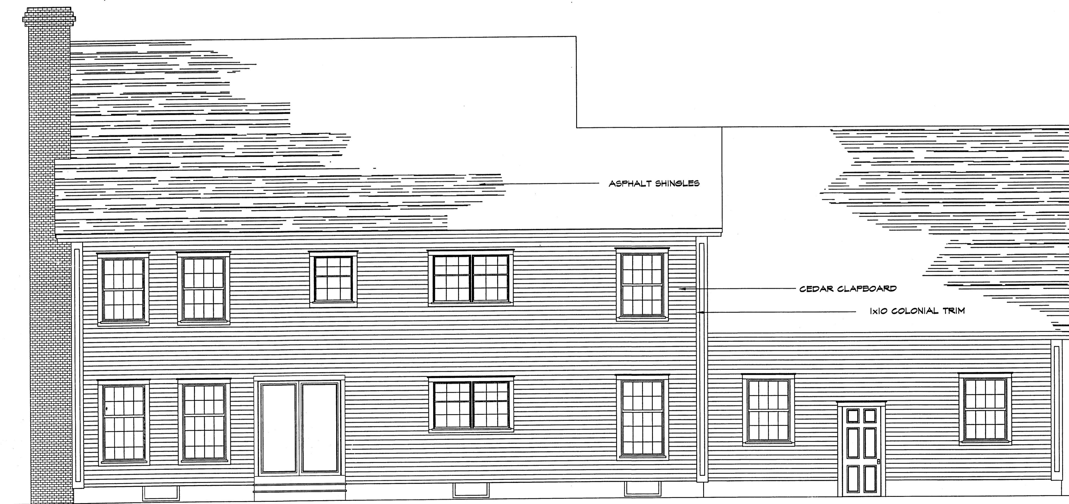
REAR ELEVATION SCALE: 1/4" = 1'-0"
