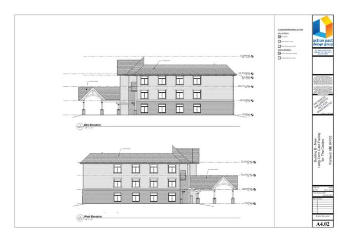
From the front building elevation, it is difficult to determine what type of roof is shown. However, from the East and West elevations above, you can see that the mansard roof is a roof element that stops and does not slope to a peak as in a typical pitched roof.
