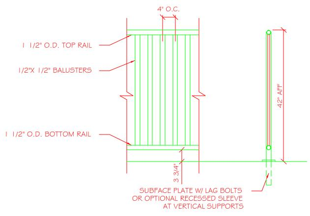
NOTE: 1 1/2" O.D. INTERMEDIATE VERTICAL SUPPORTS AT 6'-0" O.C. MAX.
