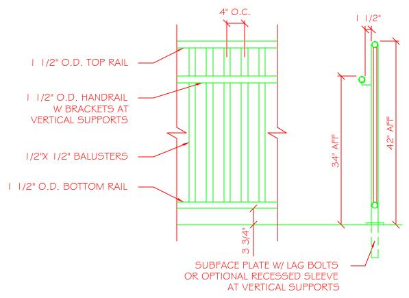
NOTE: 1 1/2" O.D. INTERMEDIATE VERTICAL SUPPORTS AT 6'-0" O.C. MAX.
