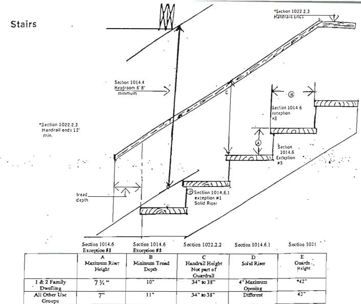
\*Guards along open-sided floor areas and along stairs located less than 30 lackes (762mm) above the floor or grade below shall not be less than 36 lackes (914mm) in height.
