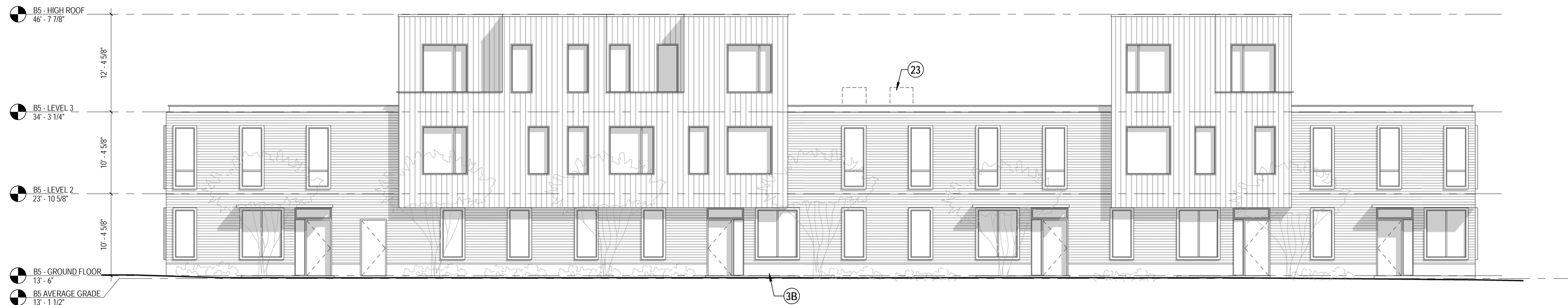
4 BUILDING 5 - NORTH ELEVATION 1/8" = 1'-0"
