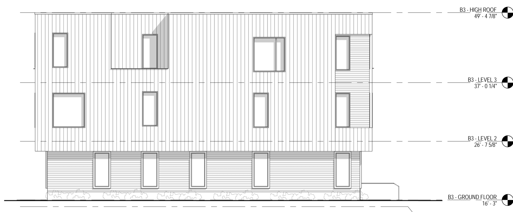
2 BUILDING 3 - NORTH ELEVATION 1/8" = 1'-0"
