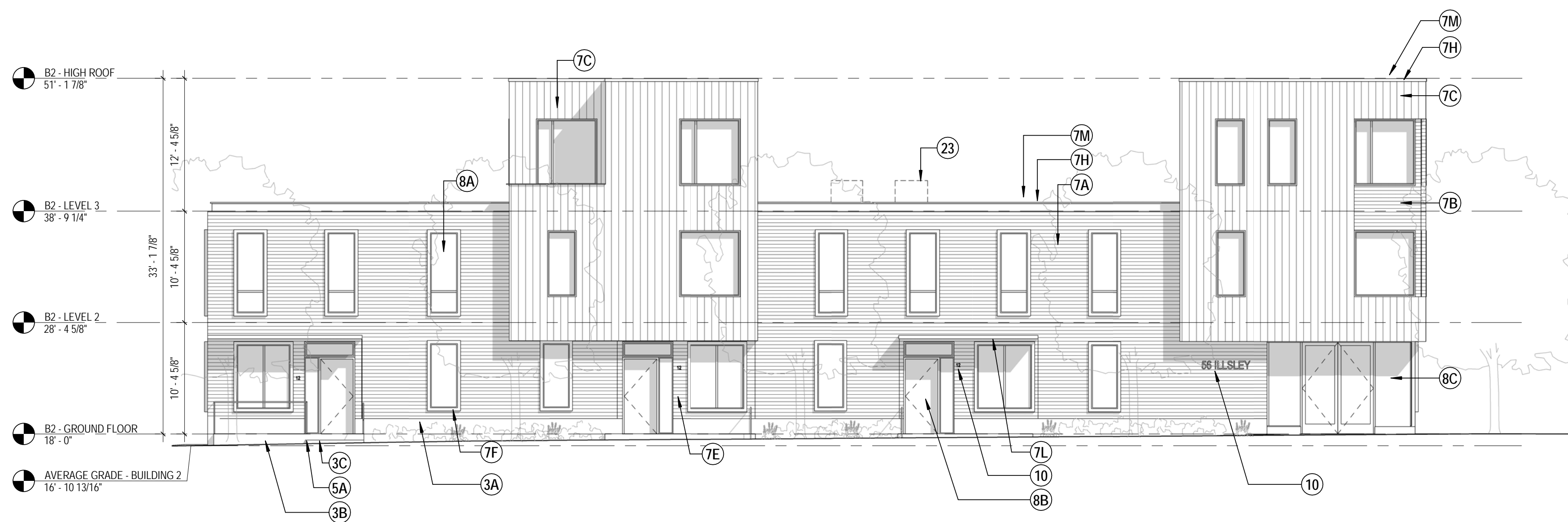
3 BUILDING 2 - NORTH ELEVATION 1/8" = 1'-0"
