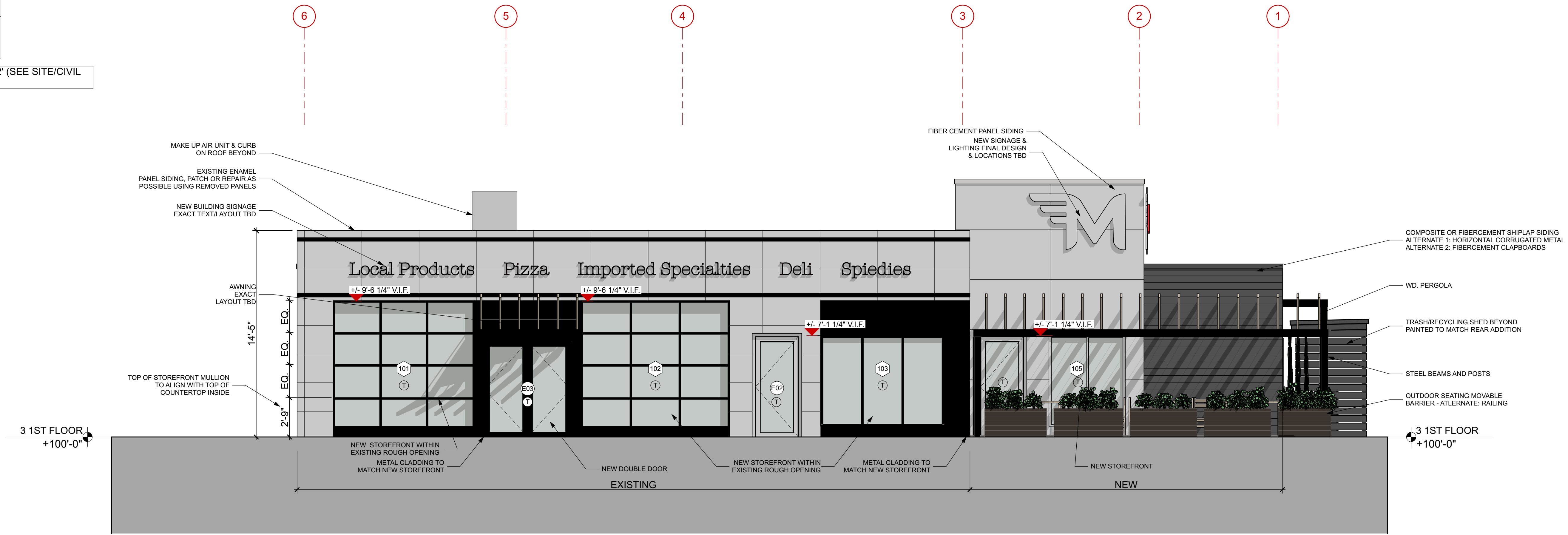
1 BUILDING ELEVATION - NORTH SCALE: 1/4" = 1'-0"
