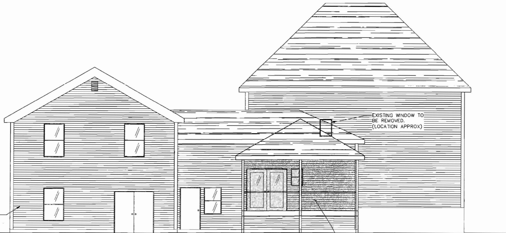
2 A-1 SOUTH ELEVATION SCALE: 1/4" = 1'
