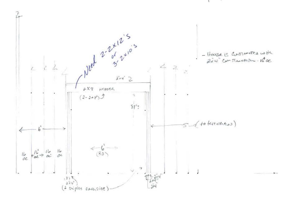
\* WALL Section IN DINING / Ketara AREA This DOOR WILL be A Slipee Type Door Insulfices of eving to Proposes Deck that will be Atlacked to the House.
