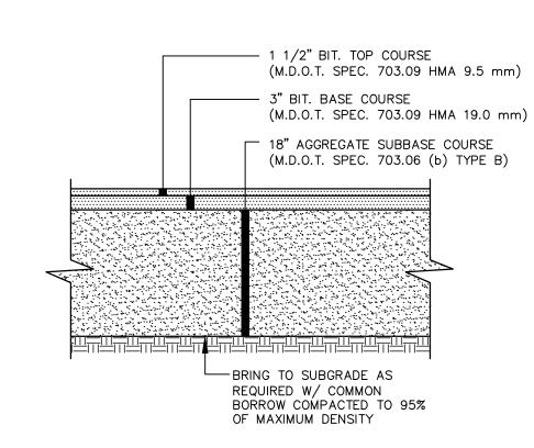
1. COMPACT GRAVEL SUBBASE AND BASE COURSES TO 95% OF MAXIMUM DENSITY USING HEAVY ROLLER COMPACTION.
