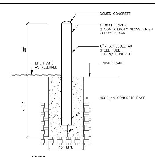
BOLLARD SHALL BE: 36" HEIGHT, STEEL PAINTED BLACK WITH REFLECTIVE STRIP, OR APPROVED EQUAL.
