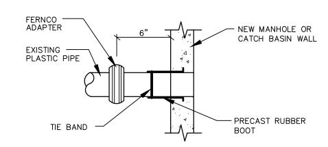
METHOD 1- EXISTING PIPE INTO NEW STRUCTURE
