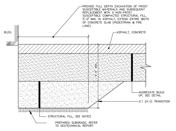
REFER TO DETAILS FOR PAVEMENT AND CONCRETE SECTIONS FOR NEW BUILDING AREAS. . PROVIDE FULL DEPTH EXCAVATION OF FROST SUSCEPTIBLE MATERIALS AND SUBSEQUENT REPLACEMENT WITH A NON-FROST SUSCEPTIBLE COMPACTED STRUCTURAL FILL. STRUCTURAL FILL DEPTH SHALL BE MIN. 4.5' FROM FINISHED GRADE. REFER TO GEOTECHINCAL REPORT.
