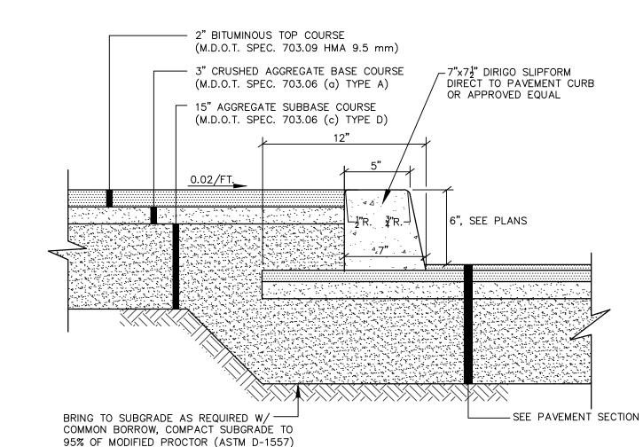
1. COMPACT GRAVEL SUBBASE AND BASE COURSES TO 95% OF MAXIMUM DENSITY USING HEAVY ROLLER COMPACTION.
