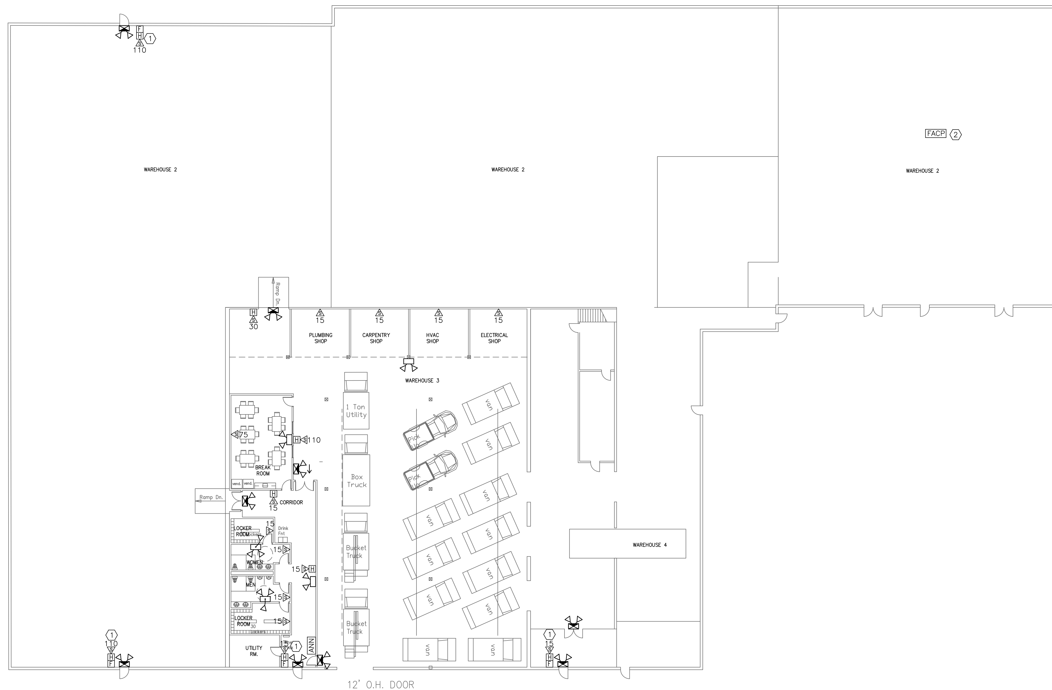
1 FIRE ALARM AND EMERGENCY LIGHTING PLAN SCALE: 1/16"=1'
