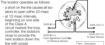
Not Used DATA IN/OUT (+) DATA IN (-) Not Used Not Used DATA OUT (-)
