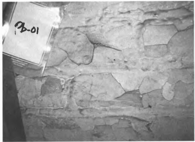
Interior basement brick wall paint chip sample, testing 3.9% lead by weight
