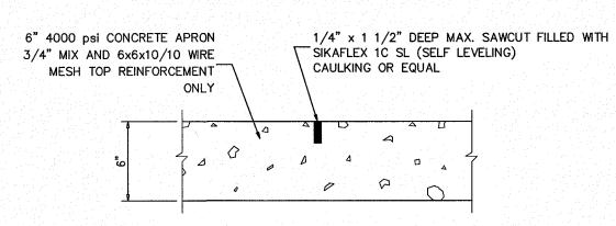
LOCATE SAW CUTS AS SHOWN ON "DISPENSER APRON PLAN" 09 TYPICAL SAWCUT DETAIL CFG12.0 SCALE: NOT TO SCALE
