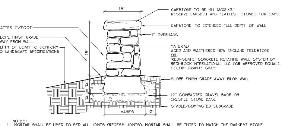
1. MORTAR SHALL BE USED TO BED ALL JOINTS (RECESS JOINTS). MORTAR SHALL BE TINTED TO MATCH THE DARKEST STONE COLOR. CLEAN ALL MORTAR FROM EXTERIOR SURFACES, NO MORTAR SHALL BE VISIBLE. TOP JOINTS FLUSH. AVOID REGULAR COURSING. FOLLOW GENERAL RULE OF ONE OVER TWO, TWO OVER ONE.
