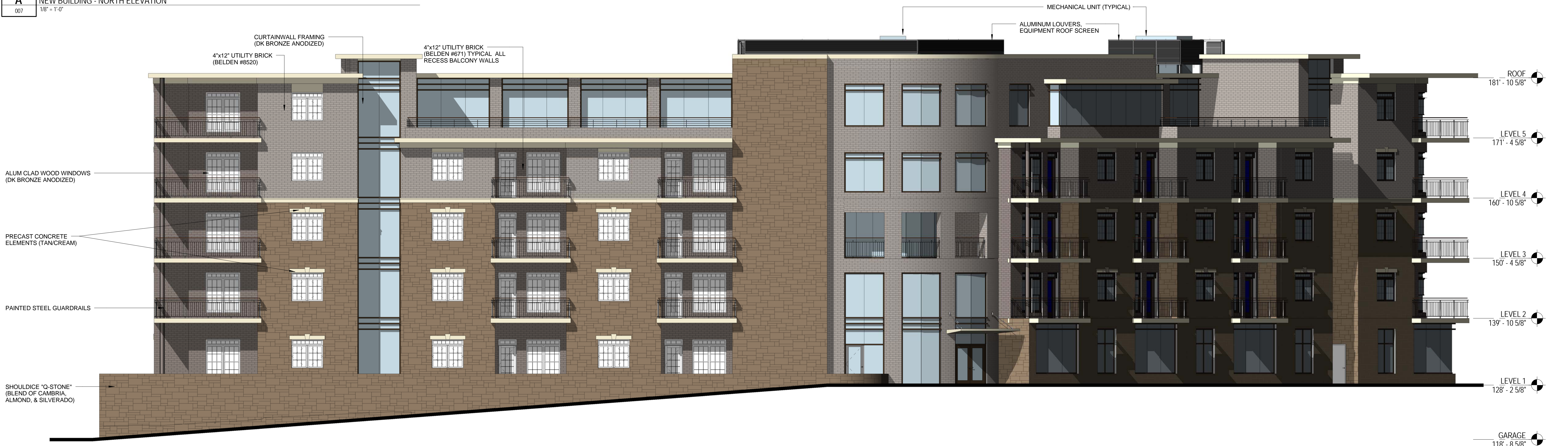
B NEW BUILDING - NORTHEAST ELEVATION 007 1/8" = 1'-0"
