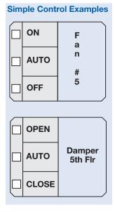
The fifth module is very adaptable to system requirements for audio or remote equipment control. Each module contains 18 LEDs and 18 switches. Each group of three switches has a latching-interlock to support operations that must be kept separated. The interlock is under software control so only one switch is active at a given time. EST3 software makes meeting the wide variety of applications needed with today's codes and building system operations easy.
