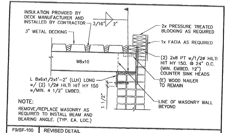
(2) 2x8 PT w/1/2ø HILTI HIT HY 150. @ 24" O.C. (MIN. EMBED, 12") COUNTER SINK HÉADS 2X PRESSURE TREATED **BLOCKING AS** 3" METAL DECK REQUIRED SEE PLAN -1x FACIA AS CONT. 3/8"x0'-10" BENT REQUIRED PLATE W/1/2" & HILTI HIT HY 150 @ 32" O.C. w/MIN. 4 1/2" EMBED.
