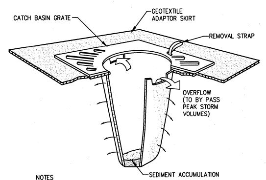
1. CATCH BASIN PROTECTION TO BE "SILTSTACK" (BY ACF ENVIRONMENTAL) OR "STREAM GUARD" (BY FOSS ENVIRONMENTAL SERVICES).
