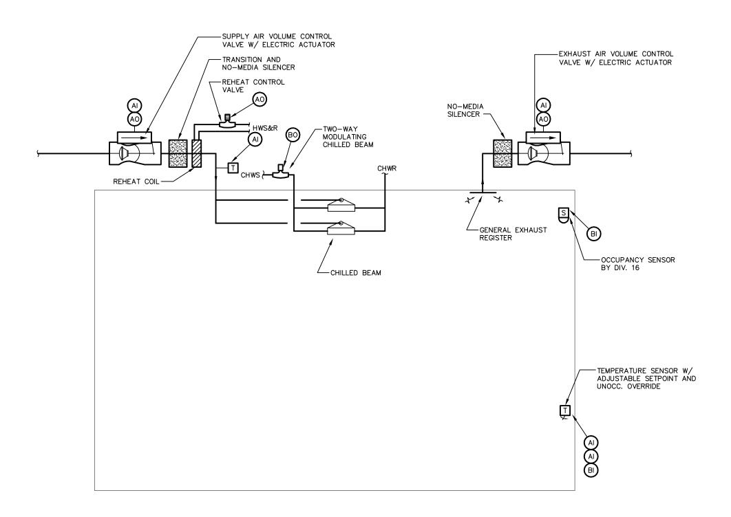
TYPICAL LABORATORY SUPPORT CONTROL DIAGRAM
