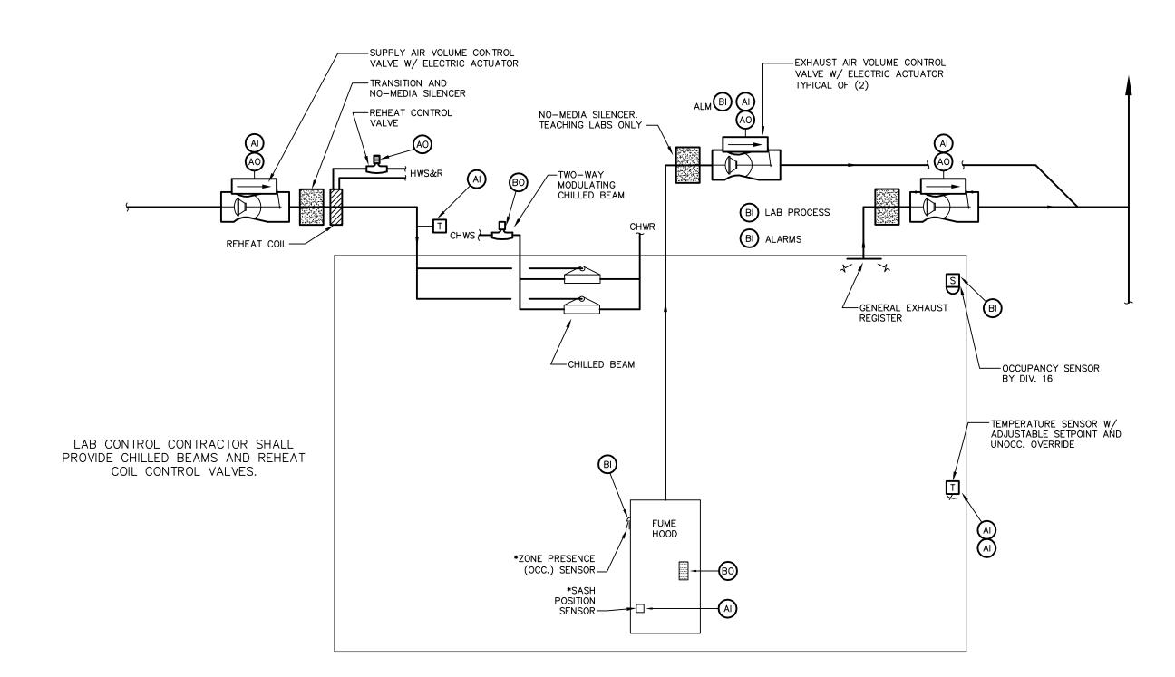
TYPICAL LABORATORY CONTROL DIAGRAM
