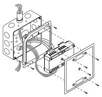
**SIGA-MCC1S:** mount the UIOxR motherboard inside a suitable Edwards enclosure with screws and washers provided. Plug the module into any available position on the motherboard and secure the module to the motherboard with the captive screws. Wiring connections are made to the terminals on the motherboard (see wiring diagram). UIOxR motherboard terminals are suited for #12 to #18 AWG (2.5 mm<sup>2</sup> to 0.75 mm<sup>2</sup>) wire size.
