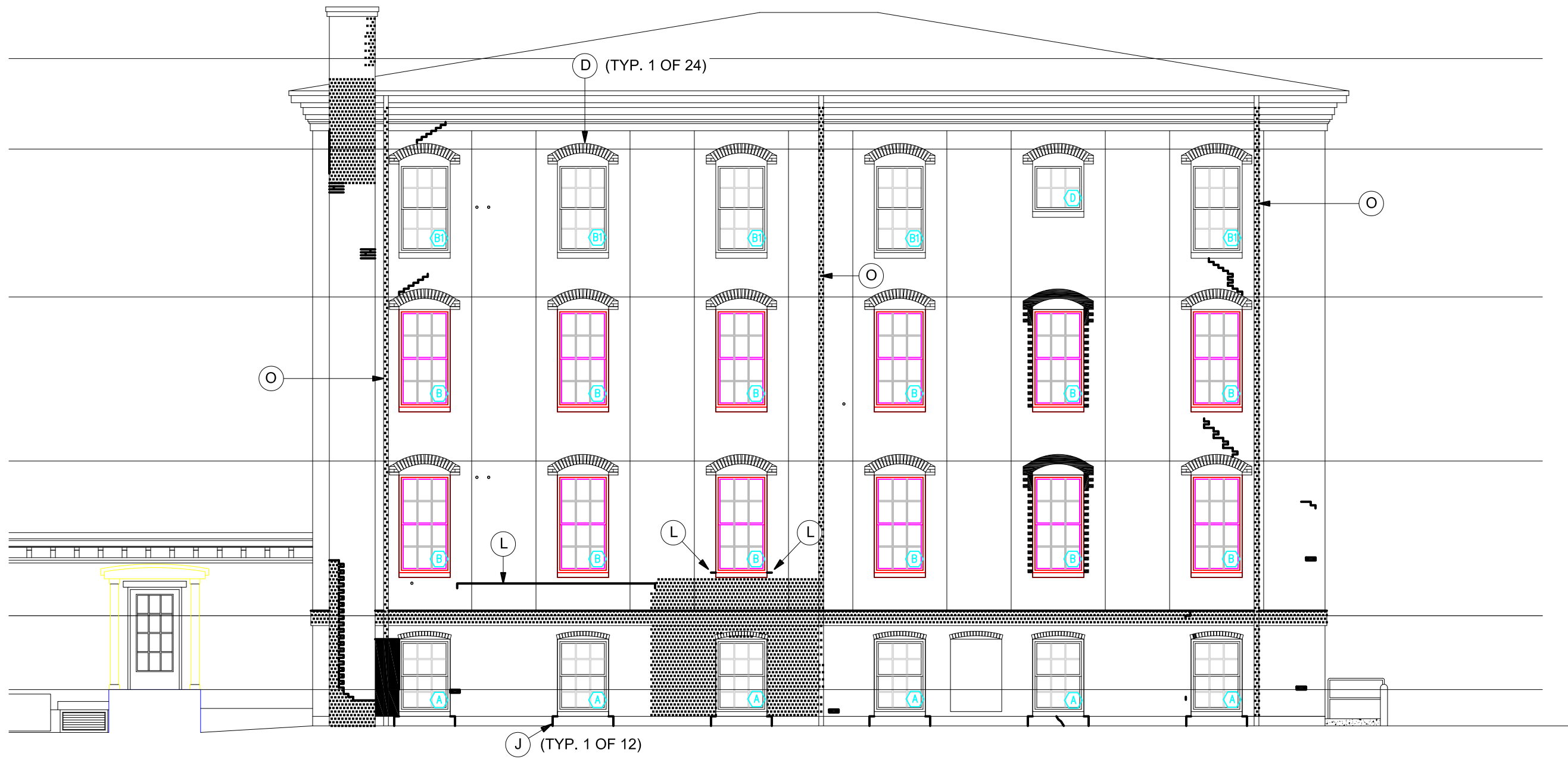
1 MASONRY RESTORATION AT SOUTH ELEVATION B1.3 1/8" = 1'-0" SEE SHEET B1.0 FOR KEY NOTES AND GENERAL NOTES
