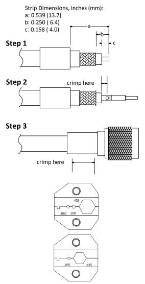
**Step 3**: Install cable assembly into body assembly so inner ferrule portion slides under braid, Push cable assembly forward until contact snaps into place in insulator. Slide outer ferrule over braid and up against connector body. Crimp outer ferrule using Die Set Cavity specified above.
