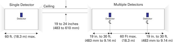
Detector positioning shown here is recommended for protected areas with flat ceilings. Spacing may vary for areas with high or sloped ceilings. In such cases, verify operation with smoke tests. In some cases potential smoke layering may be overcome by installing multiple beam detectors at different heights.
