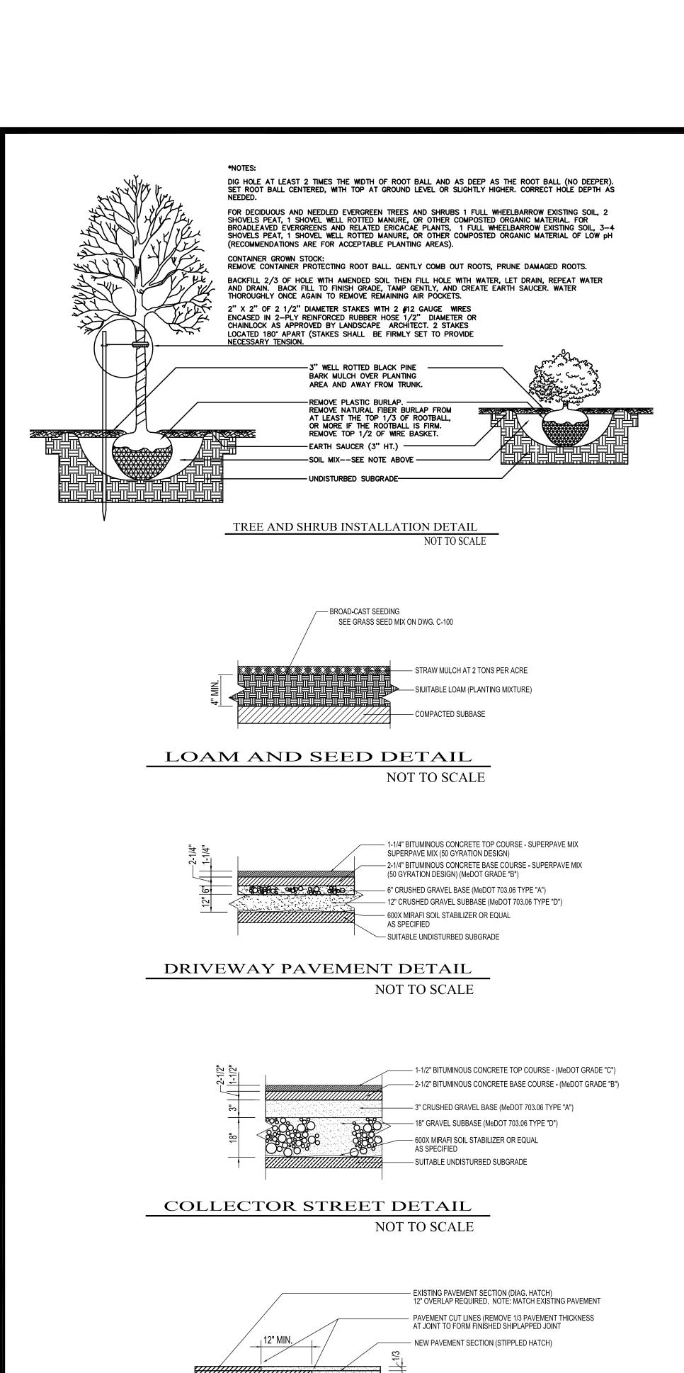
(EXTEND 3 FT. MIN. BEYOND SIDEWALK LIMITS) 2" CRUSHED GRAVEL BASE (MeDOT 703.06 TYPE "A") (95% COMPACTION - SEE PROJECT MANUAL)
