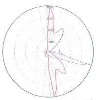
Maximum candé a = 13705 34. Located at Horizontal Angé a = 85, Vertical Angé a = 70. Vertical Plane Thiough Horizontal Angé a (85–265) (Thiough Max Cd) - BLUE Horizontal Cone Through Vertical Angé a (72) (Through Max Cd) - PBD
