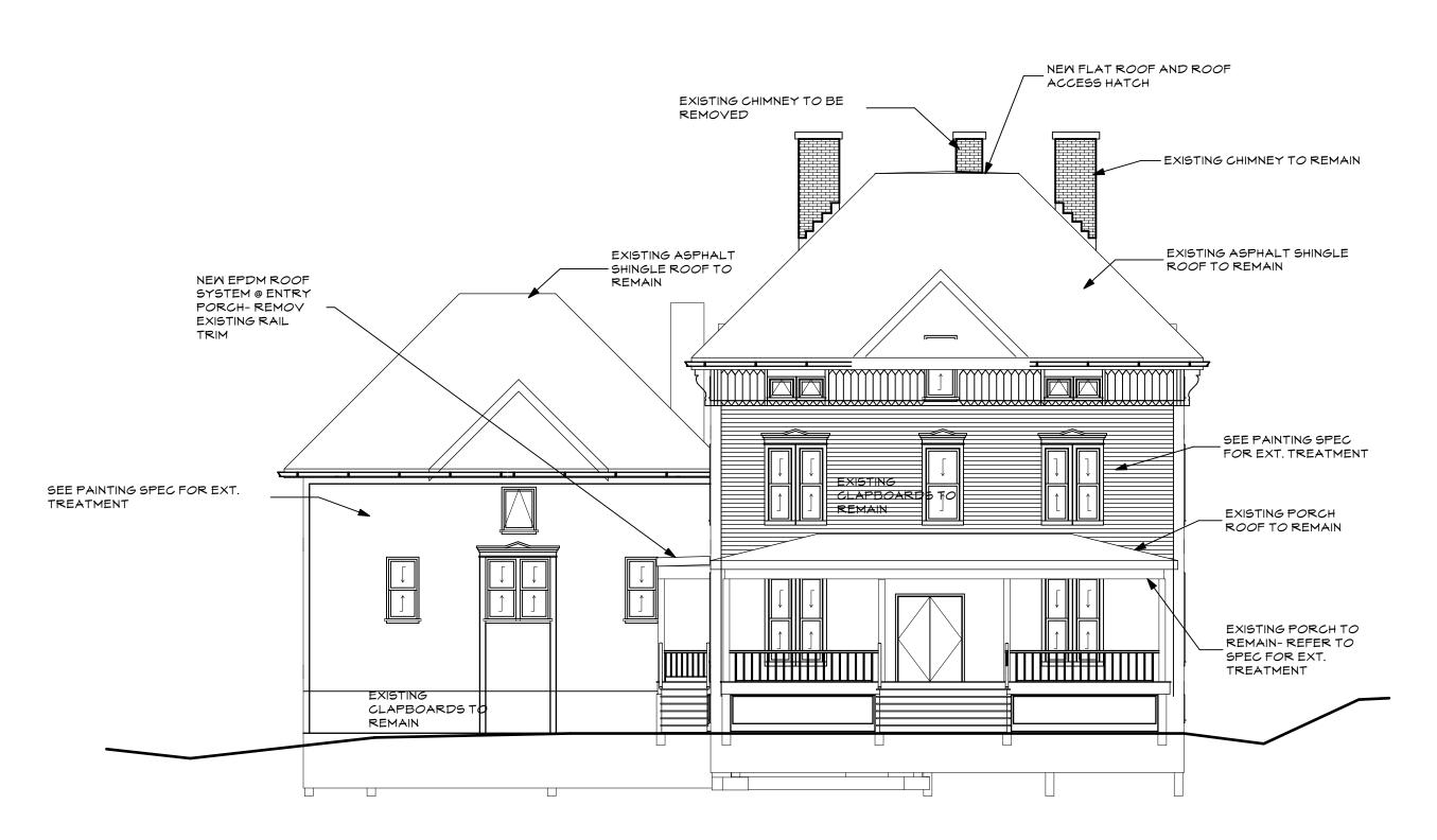
1 Left Elevation A2.2 SCALE: 1/8" = 1'-0"
