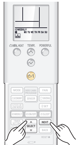
The program and day of the week / “NO TU WE TH FR SA SU” will be flashing
