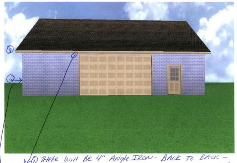
LD THERE WILL BE 4" ANGLE IRON - BACK TO BACK over Doorway- They will Extend 8" on each enD - AND THE BLOCK WILL be Filled Solid WITH CONCRETE -I every 5 courses of BLOCK WIll Have steel sheets of Durwall Incorperated into mortan Joints For 3 Roof Will have 24" wide trusses - every 2ft. STRENGHH -
