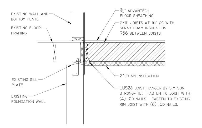
Typical Floor Framing Detail at Existing
