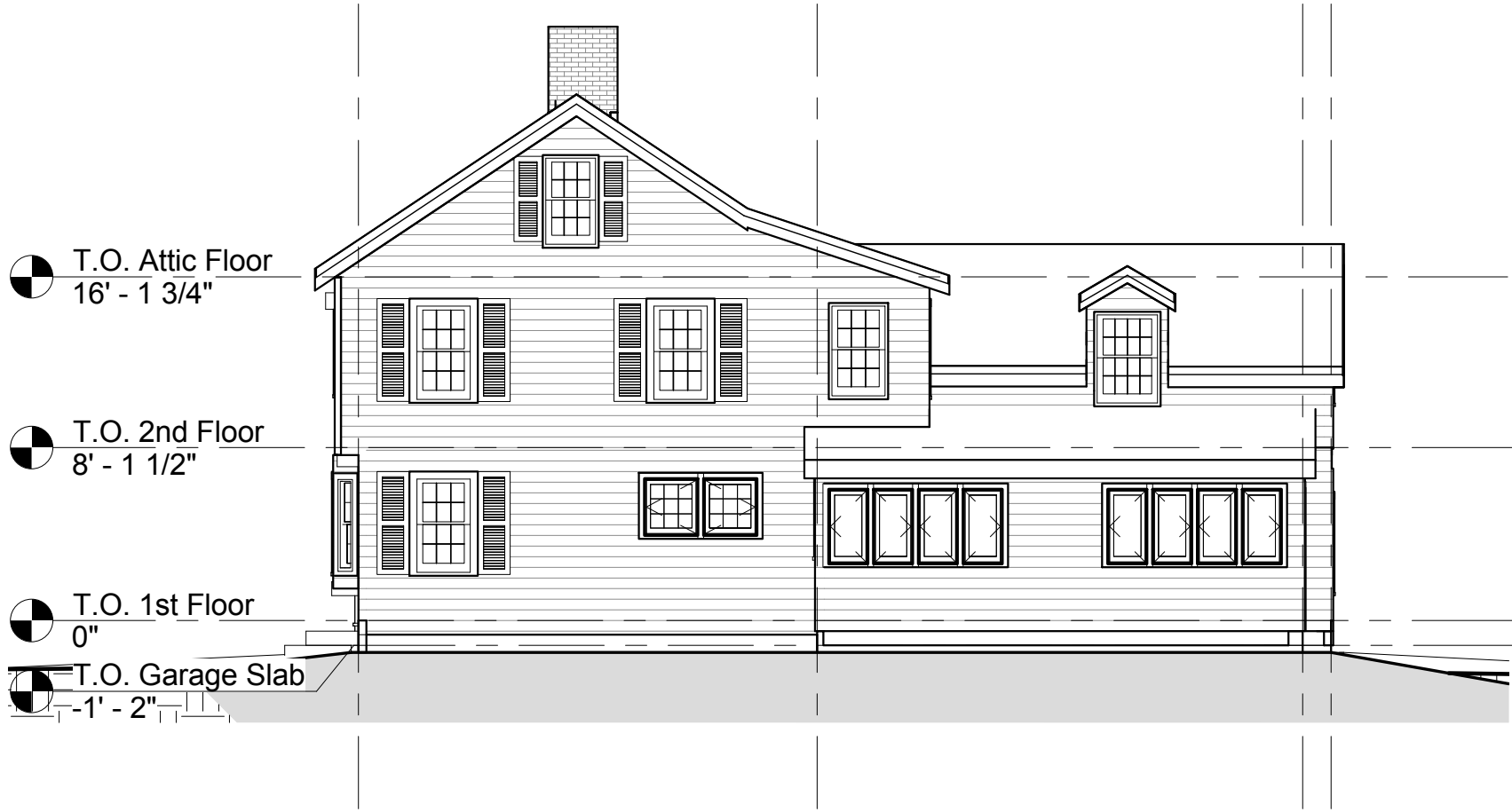
1 Existing Elevation - Side 1/8" = 1'-0"
