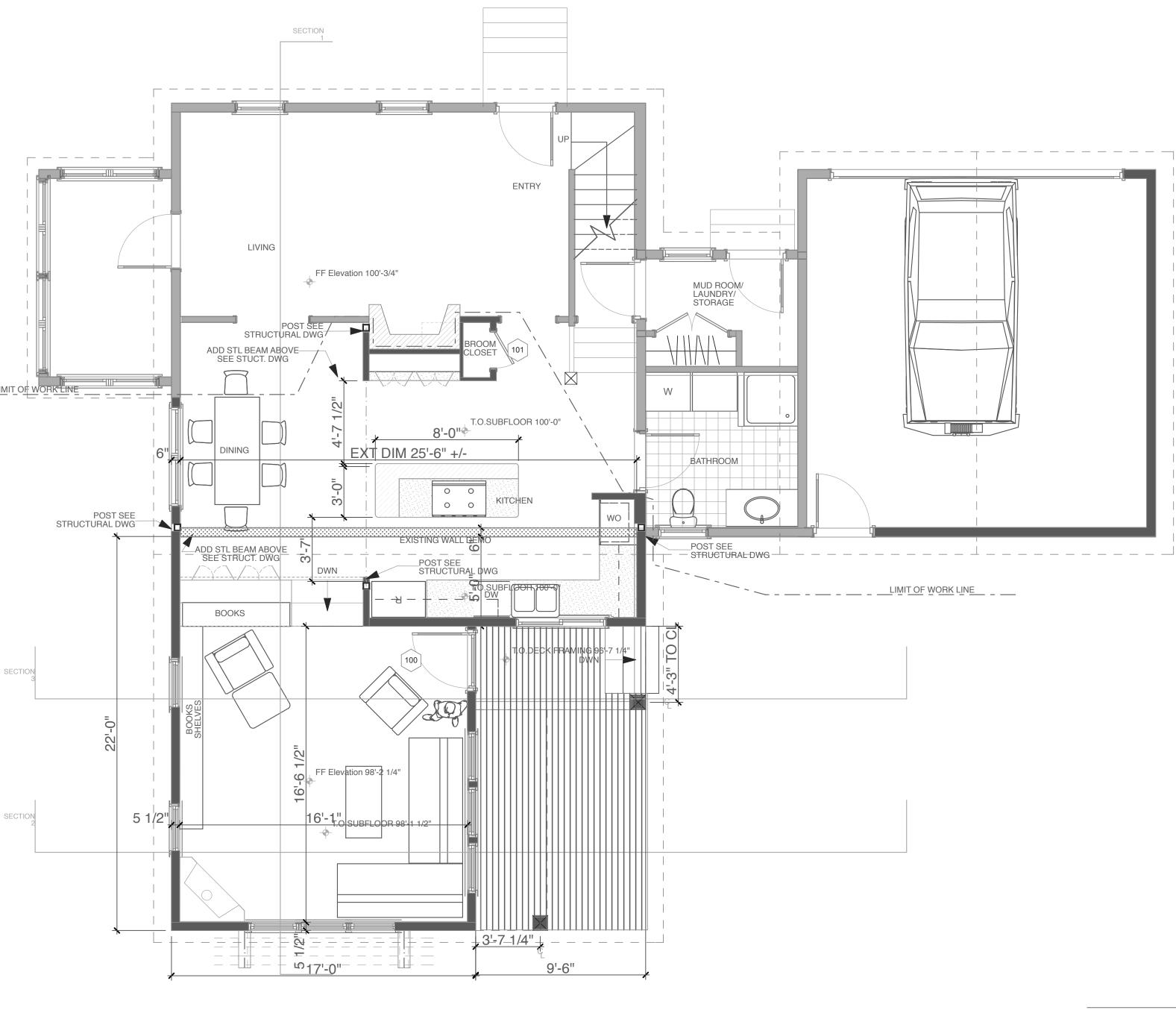
1st Floor Existing Plan **Proposed 1st Floor Plan Addition** 1/4" = 1'-0" 1/4" = 1'-0"
