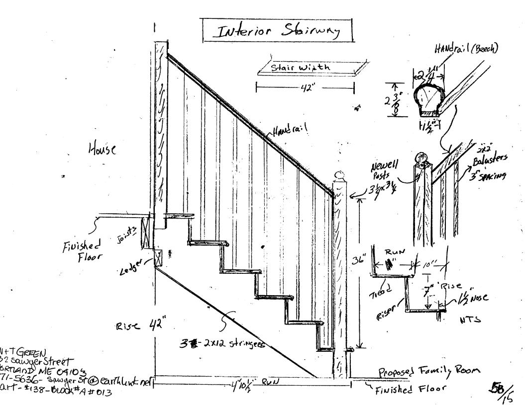
Stairs Interior Treads and Riser's 1. Junished Floor to finished floor 42" ~ D We 71/2" Lusers 1/4"
