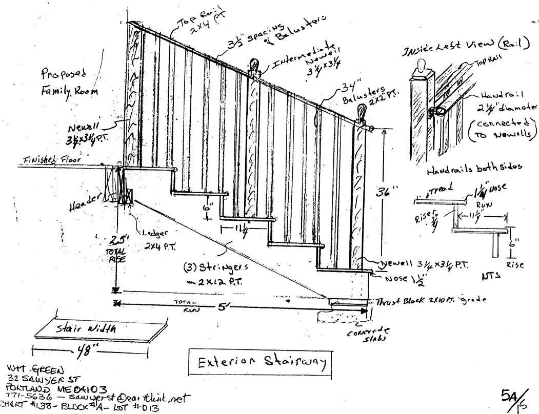
Stairs - Exterior TREADS - RISERS 1. Finished floor to grade = 30" @ use 6" tusers = 30" = 5 suis 10 treads = 5# tread weaths = 11/4"
