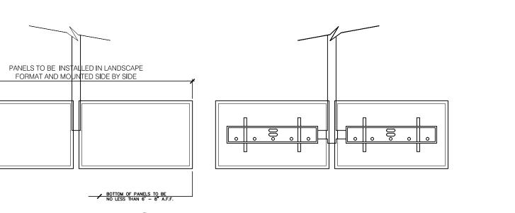
6 MENU BOARD BRACKET DETAIL SCALE: 1/2" = 1'-0"
