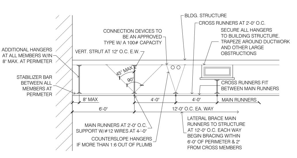
SUSPENDED CEILING DETAIL NOT TO SCALE
