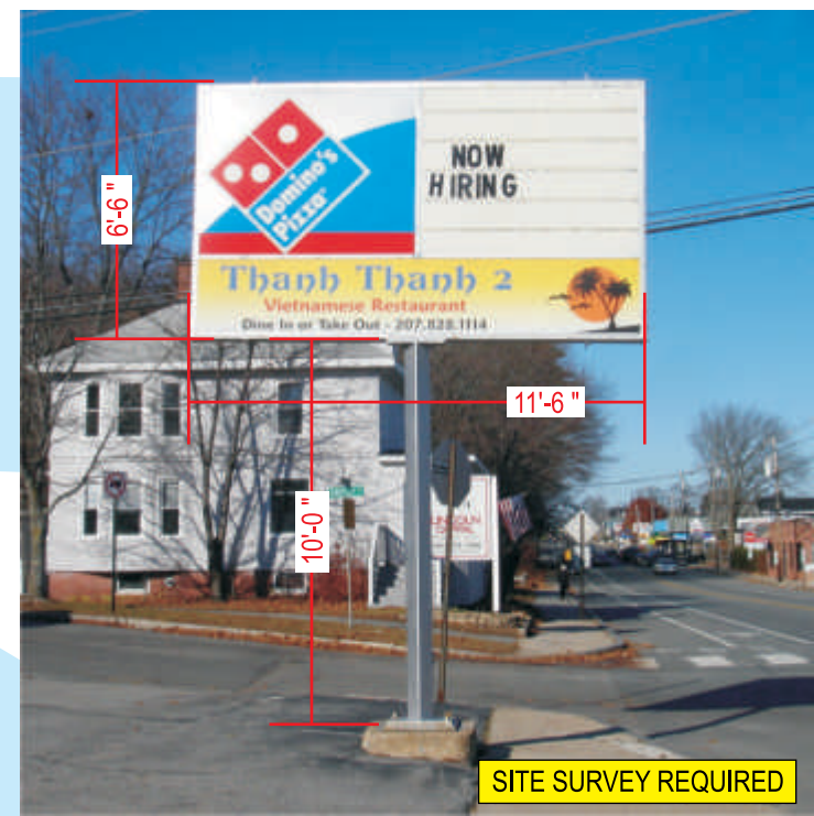
CURRENT SIGN ELEVATION / SCALE 3/16"=1'-0"
