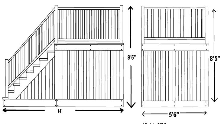
Stairs: 7" rise 10" tred (4' total length) Railings: 3%" tall (running at a 45^ angle) Horizontal Rail: 3%" x 10' (Hight Measurement from ground level)
