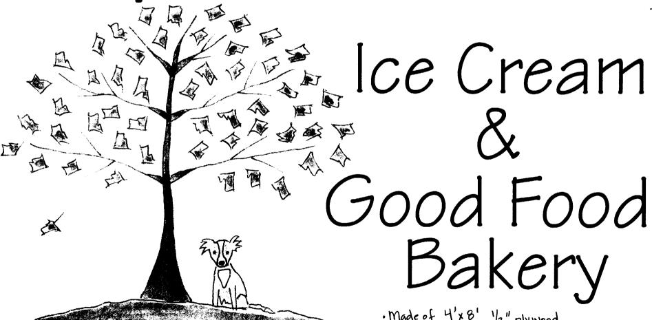
· Made of 4'x8' 1/2" plywood · mounted on 2 posts secured > 48" in ground 5 posts held pre existing signage
