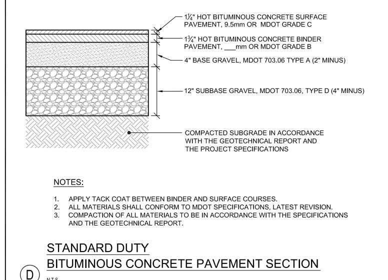
1" HOT BITUMINOUS CONCRETE SURFACE PAVEMENT, 9.5mm OR MDOT GRADE C
