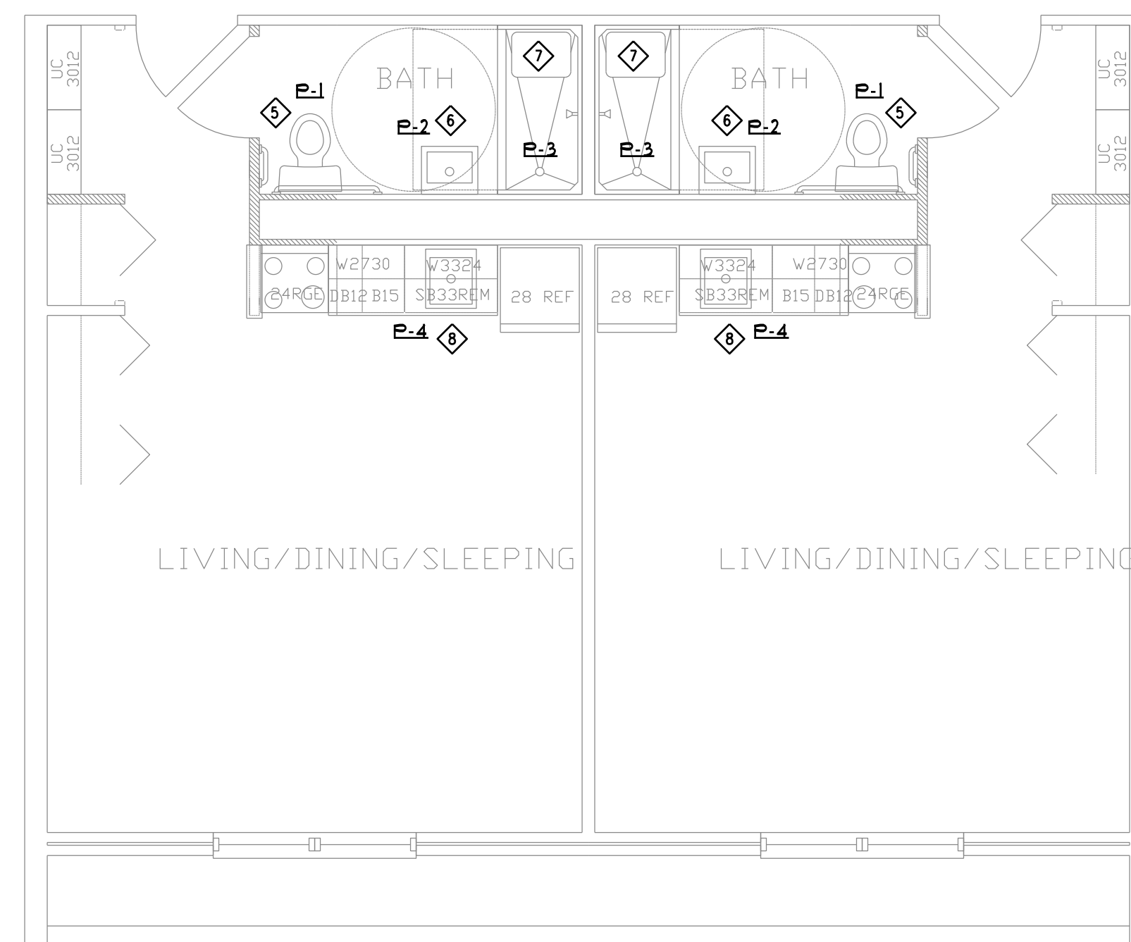
UNIT PLUMBING PLAN SCALE - 1/4" = 1'-0"
