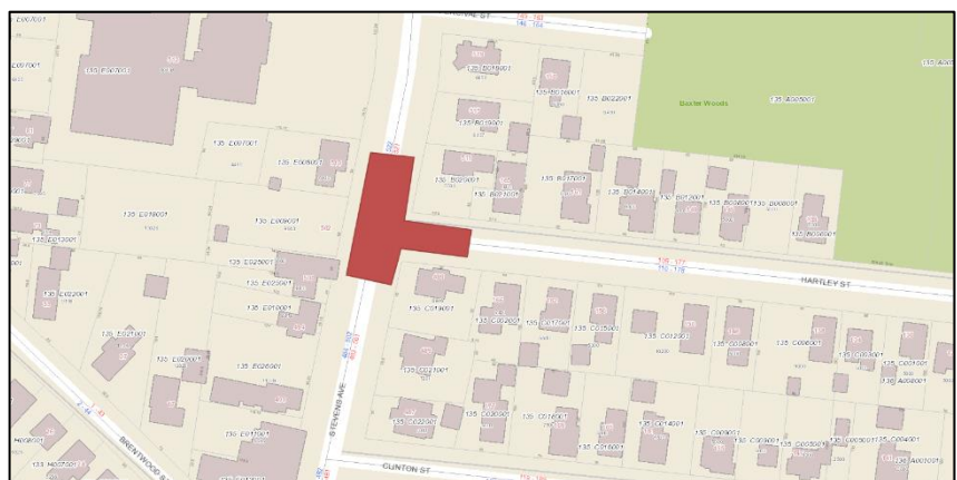
Figure 4: Area of constriction shown in red, resulting from vehicles entering/exiting Hartley Street simultaneously
