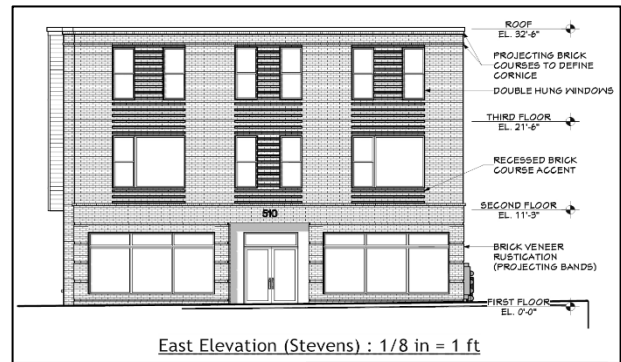
Figure 6: Stevens Avenue elevation (front)
