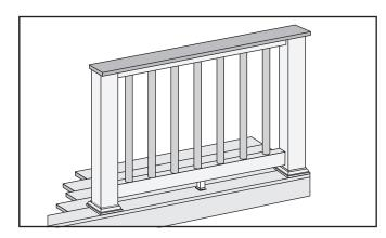
**Important: ONLY** use for use with pressure treated 4x4 post (3.5" nominal square) and 4" x 4" (102 mm x 102 mm) post sleeve. Trex Post Mounts or Joist Mount Posts cannot be used with Select Cocktail railing.
