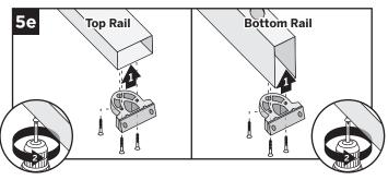
5e. On the TOP RAIL, attach the assembled bottom stair bracket to the side with baluster holes. On the BOTTOM RAIL, attach the assembled bottom stair bracket to the OPPOSITE SIDE of the baluster holes. Attach both brackets using three #8-18x1" self-drilling screws (provided).
