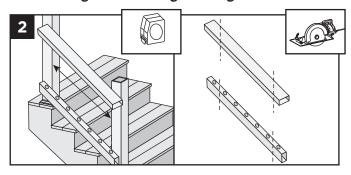
2. Set railing along the nose of the stair treads, making sure baluster holes are vertically aligned and mark line at each intersection. When measuring, cut equal lengths from each side of railing allowing a minimum of 2" on each end from the last baluster hole to the end of the rail. This will ensure proper baluster and bracket placement and equal spacing of balusters per each railing section.
