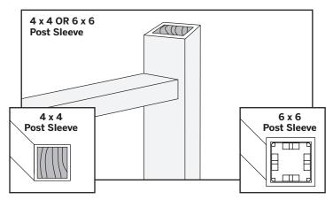
Both 4" x 4" (102 mm x 102 mm) or 6" x 6" (152 mm x 152 mm) post sleeves work well for angles up to 45 degrees. Bottom rail brackets may
