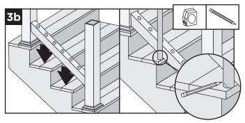
3b. Set bottom railing on nose of stair treads and set baluster at 90° on the outside of the railing, mark and measure the angle.
