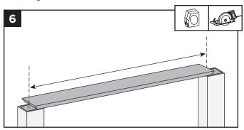
6. Cut deck boards to appropriate length of railing span, remembering to include extra space on each side of the deck board to allow for attachment to the post. Decking boards must cover 1/2 of the pressure-treated post to allow this to be fastened later.
