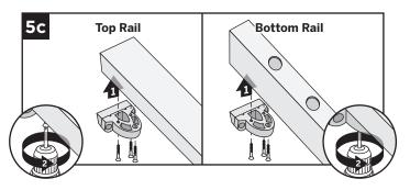
5c. On the TOP RAIL, attach the assembled top stair bracket to the side with baluster holes. On the BOTTOM RAIL, attach the assembled top stair bracket to the OPPOSITE SIDE of the baluster holes. Attach both brackets using three #8-18x1" self-drilling screws (provided).
