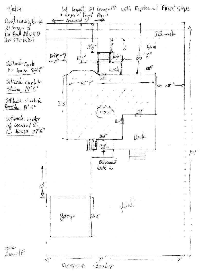
21 Leonard St Front purch + Stairs framing layout 7/10/04 David + Laura Burke 21 Leonard St. Portland ME04/03 Top View 207 773-6067 Abuse 15 Posis 4x4 x8, times ente ledgen 2x6x12 Pt 1 ft 16 Frame 2x6 11/ Joist 2x6 1 6 Beam Beam 2x 12x12 Ril 1 sts 4x4 townedspindle Decking 5/4 ×6 × 12 Pt Hand Rails modeled 2x4 pt Spindles a apart Scale: Spirt  $\frac{1}{2}u = 1$ Strips ripped from a 4 pt 3" thick " Spacing facio INOP Step have on somation of deep content
