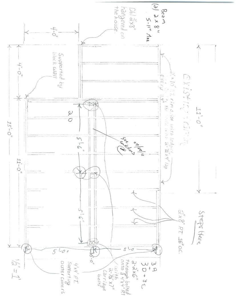
Where 4"X4" Support Posts do not sit on existing slab, they will sit on a lo" soma tube with a 2' Big foot base filled with Concrete Set at 4' below prade.
