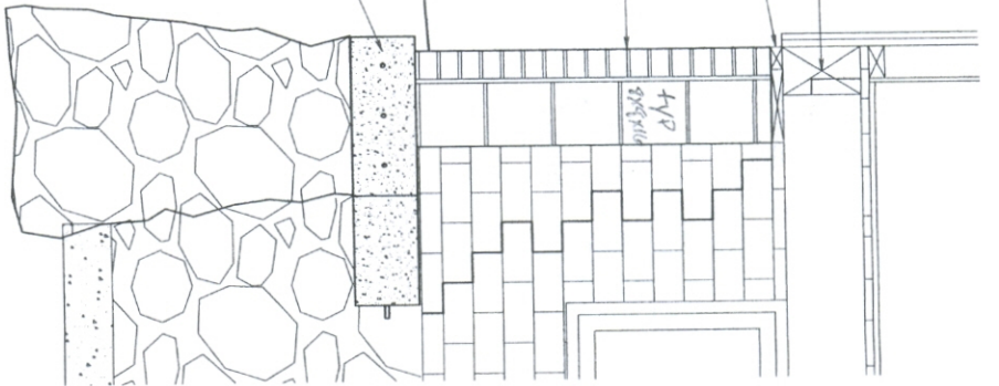
Section showing repairs to existing foundation on left side of building scale 1" = 1'
