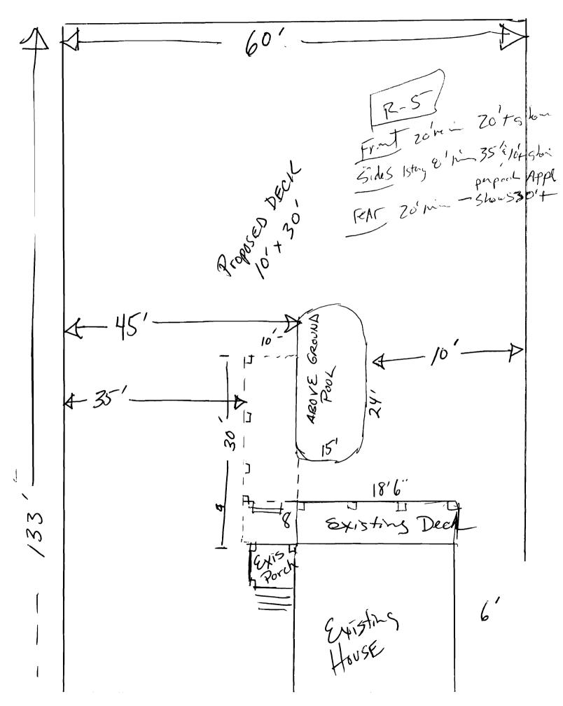
P.T. 2×6 Floor joist 160.C. 8/8" Sonotubes dug 4'deep spaced 8-10 TBAIF. 7 or 8 stairs is me. to Jw. + - 10" Above Ground 48" high ZHISYAS self closing gate 2 deck approx. 56"high 30 Self closing gate 1(48" high) 2 STORY Existing 8' x 18'6" DECKS handbails 36"-42" above deck -,9,6 T.B.D.I.F. deck approx. 48" Existing Single FAMILY HOUSE high
